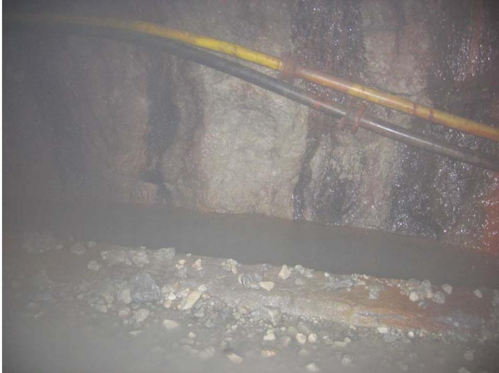
Figure 2-3 Seawater flowing into Sanshandao Mine (Source: N.Irwin)
