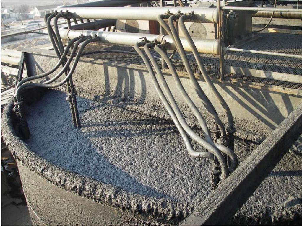
Figure 2-9 Leach Tank at MIC BioGold (Source: B.Klein)
